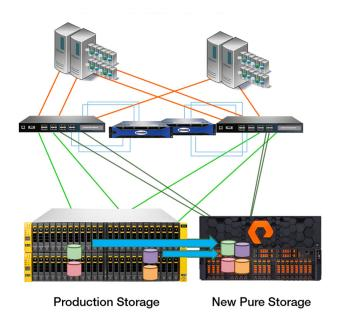
The DMS Intelligent QoS feature (iQoS) allowed the maximum use of all available bandwidth for copying data without impacting production I/O quality, automatically throttling migration when the LUN was too busy. The entire process was transparent to the database applications and caused no impact to production. At cut-over, the database owner simply unmounted the database from the old storage and remounted on the new device in a few short minutes.
